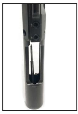
9. Push the bolt in towards the carrier until bolt rotattes and comes to a stop, then turn the bolt cam pin through 90 (i.e., at right angles to its normal position.
